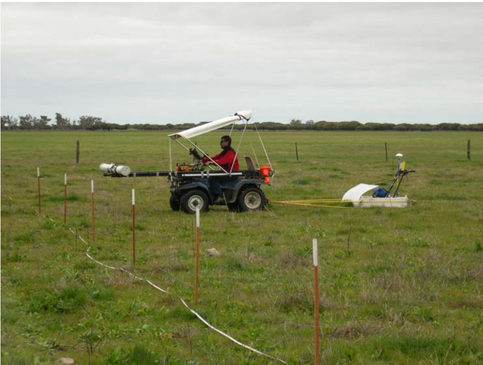
Philip Mill “Ecophyte Technologies” conducting EM and GPR surveys.
